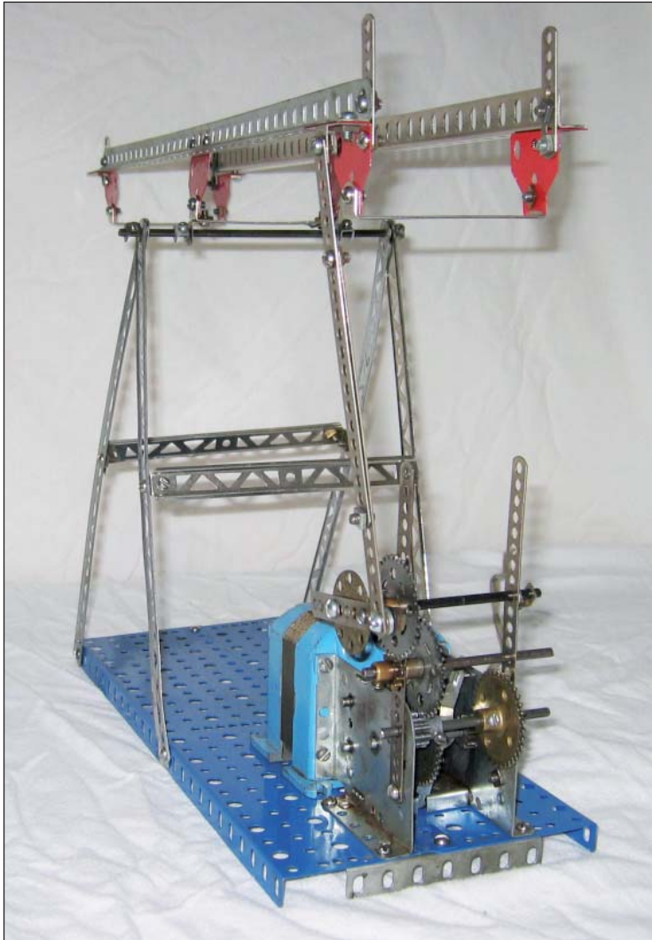
The track pivots on the main axle via 2 CH's mounted on an N (round holes of CH on the axle).
