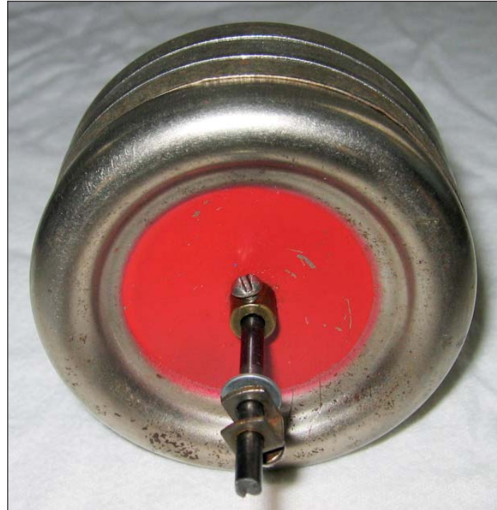
Washers on the wheel axle must be on the outsides of the rails.
